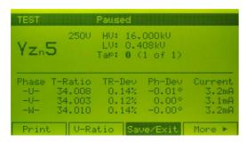
To assure the safety of the operator the TTR 2796 first applies a low test voltage to check for reversed connection and then the test voltage is applied. In "Auto Voltage" mode the test voltage is automatically set to the highest voltage possible. Or the user can choose manually between four different test voltages. After starting the test the TTR 2796 delivers results of voltage ratio, turns ratio, ratio deviation, excitation current and phase deviation within half a minute.
