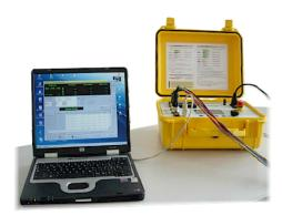
The included TTR APSW 2796 software offers remote setup and control of the TTR 2796 from a computer through a USB connection. Additionally advanced analysis is available like customized graphs, trending and report generation capabilities. Pre-captured measurements as well as live data can be analyzed, stored or recalled.
