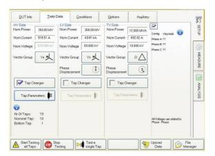
The comprehensive user interface guides the operator through the setup steps by entering nameplate info, transformer vector group, environmental conditions and user comments.
