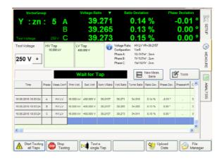
The software offers additional tools for in depth analysis of the measured transformer data. Flexible graphs allow quick comparison of several measurement series from live or precaptured data. Additional limit lines show a colourful graphical interpretation of preset margins.
