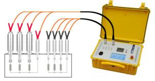
Once the cable set is connected to the test object, the instrument will automatically measure the turns ratio of all taps. Then - without reconnection - the winding resistance can be measured. Finally the demagnetization function will put the transformer in a demagnetized state. A complete transformer **can be tested by a single person** in a fraction of time compared to traditional instruments.
