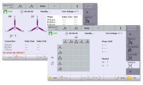
**The type detection** part of the software works as a nameplate guesser. It helps the user to determine the correct transformer configuration by showing the possible types and eliminating the wrong vector-groups during the automatic detection process.
