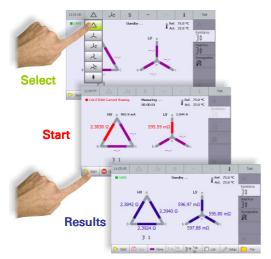
Select the test object by touching the appropriate icon and press start – the unit then visualizes each test cycle and displays the results graphically or in list format.
