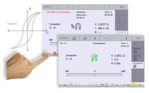
The 2293 includes a **fully automatic demagnetisation** feature which eliminates the magnetic remanence. Select the test object by touching the appropriate icon and press start – the unit visualizes the whole demagnetisation cycle and performs the correct core demagnetisation.
