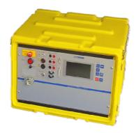
High performance is the key feature of these high current resistance meters based on the four point measuring technique. The instruments are especially designed and optimized for low resistance measurements in highly inductive circuits. The design responds to the needs of utilities and transformer manufacturers for portable unit of high accuracy and ease of operation.
