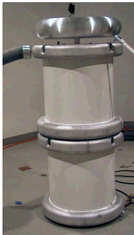
200 kV cascade with 2 PZT 100-0.1 transformers
