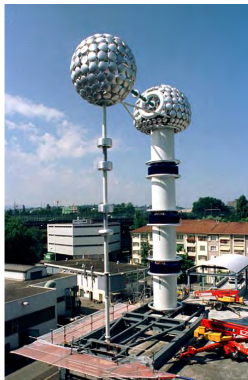
Example of 1'500 kV, 1.2 A cascade made of 4 transformers
