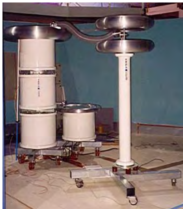
300 kV cascade with 4 PZTL 100-0.25 transformers
