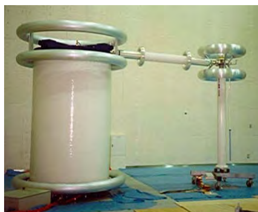
Test system 350 kV, 2 A with damping resistor
